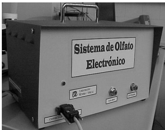
Fig.8. Photograph of the electronic nose system
